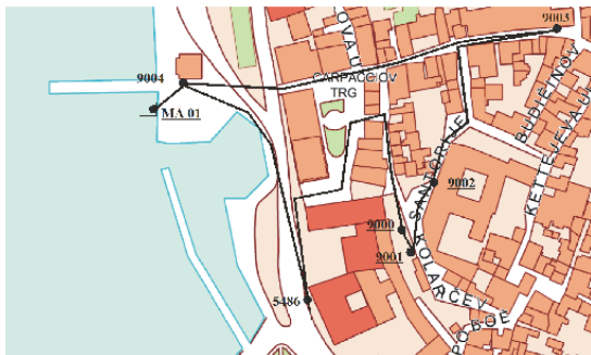
Nivelmanska mreža mareografske postaje Koper (vir: DPK-1000 GURS) Benchmarks of the tide gauge Koper (source: DPK-1000 GURS)
